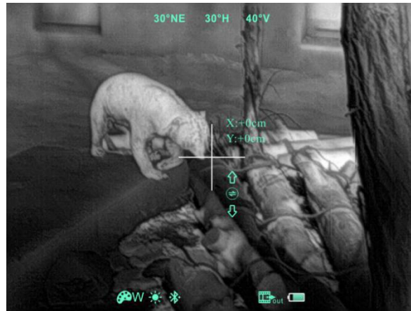
Fig. 6-6 Image calibration interface
