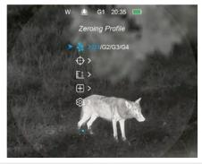
Then select the Zeroing option ( ) and short press the Menu (4) button to enter the Zeroing interface.
