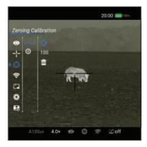
Adjust the reticent position of the selected zero distance In the reticent zeroing interface, the X/Y position Of the reticent may be adjusted to match the point of impact.
